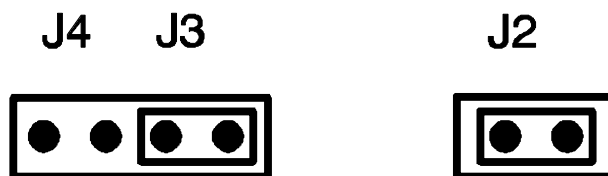
Figure 4 - 4-20mA jumper settings
